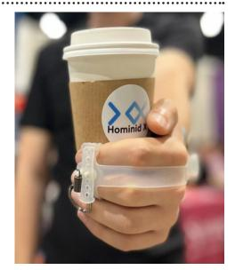
This wearable device can be easily adjusted to accommodate various hand sizes. The design functions as a supportive frame around the user's hand, aiding in the natural closure around objects. The Fiber Grasp utilizes springloaded cable mechanisms instead of costly electronic components, making it a more budget-friendly option compared to other high-end devices.
